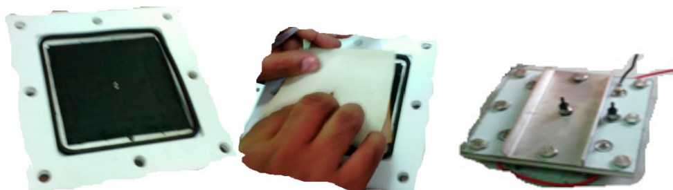
Figure 7. Assembly of two electrode sheets and membrane inside the CDI cell.
