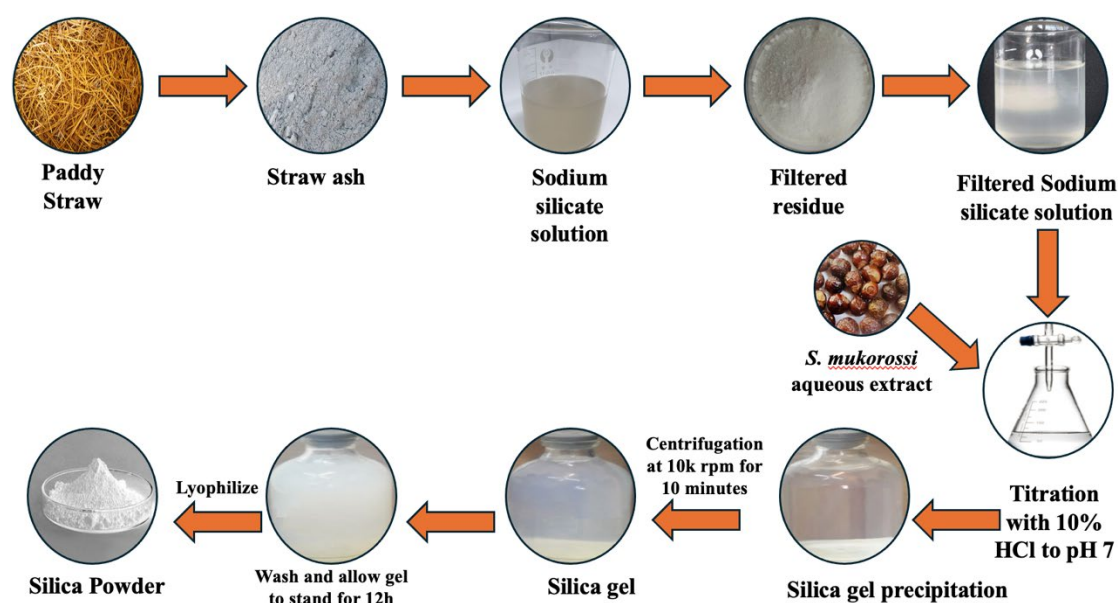
Figure 4. Schematic representation of silica nano synthesis by sol-gel method using aqueous extract of paddy straw. Adapted from 66.
