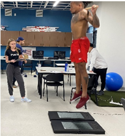
Figure 3. Countermovement jump assessment using dual uniaxial force plates.
