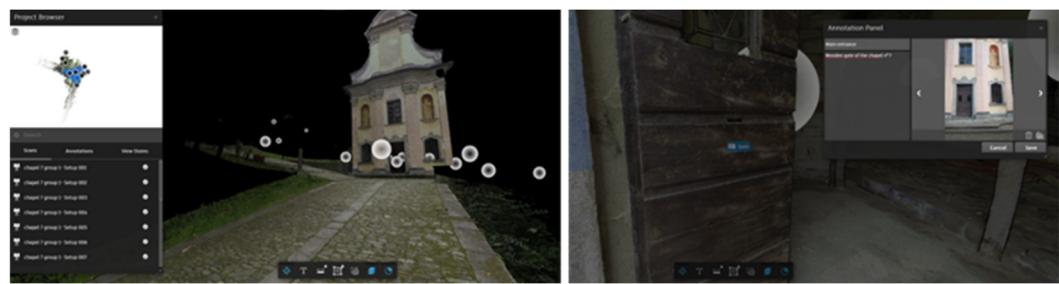
Figure 3. An example of use of the Autodesk Drive platform, showing the scan navigation of the point cloud and the use of annotation function for information and media attachment. Dataset from [64].
