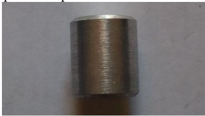
Figure 6. Compression Sample before.
