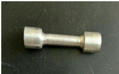
Figure 4. Tensile sample before testing.
