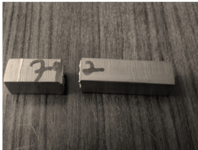
Figure 9. Impact Specimen after testing.
