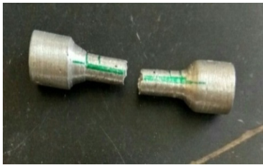
Figure 5. Tensile sample after testing.
