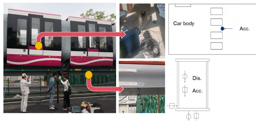
Figure 4. Layout diagram of the measuring points. For the car body, vehicle accelerations (Acc.) were tested; for the track beam, vertical displacement (Dis.), vertical and lateral Acc. were tested.
