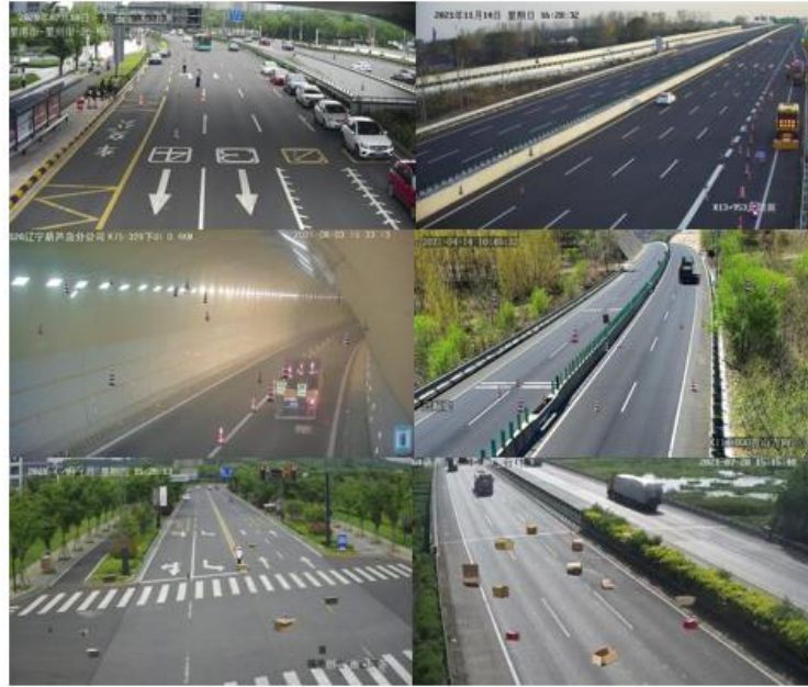
Figure 5. An example diagram of a reflective cone and sprinkles enhanced with Copy-Paste.
