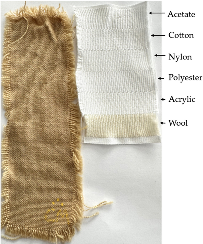
Figure 1. An example of a tested fabric with a reference multifiber fabric. The sample was dyed according to the conditions proposed in Process 2 and it is sample 3.
