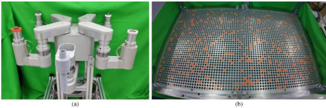
Figure 10. The robot HIT_Spibot and the real experimental tube plate. (a) HIT_Spibot. (b) the square-distributed tube plate. Due to the large size of the tube plate, the tube plate is taken with a wide-angle camera, which looks like an irregular curved tube plate, but is actually a rectangular tube plate. The orange circles are randomly added obstructed tube holes.
