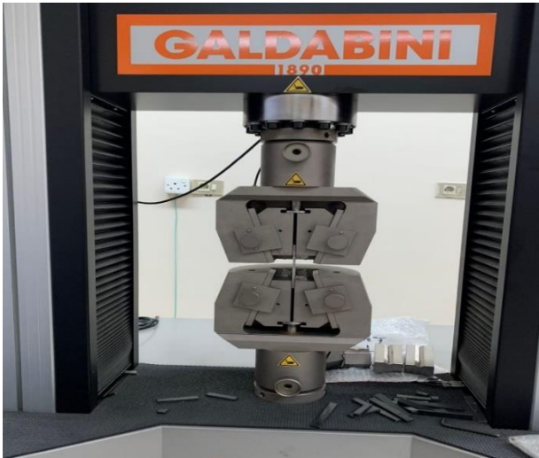
Figure 29. Tensile specimen adjusted at Tensile Testing Machine.
