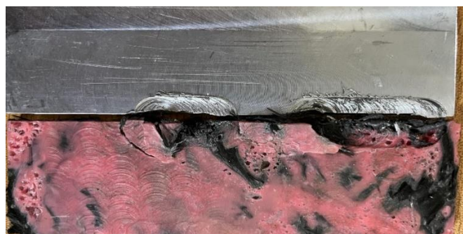
Figure 6. FSW of composite plate from Iso thermal heat press with aluminum.
