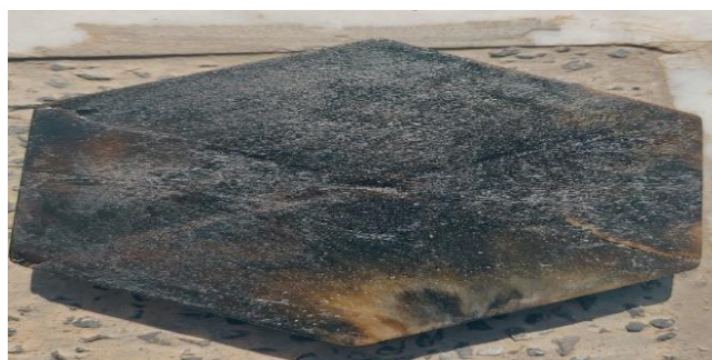
Figure 4. ABS and carbon fibers through Thermal process.
