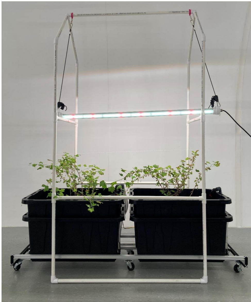
Figure 8. PVC + mobile platform structure .
