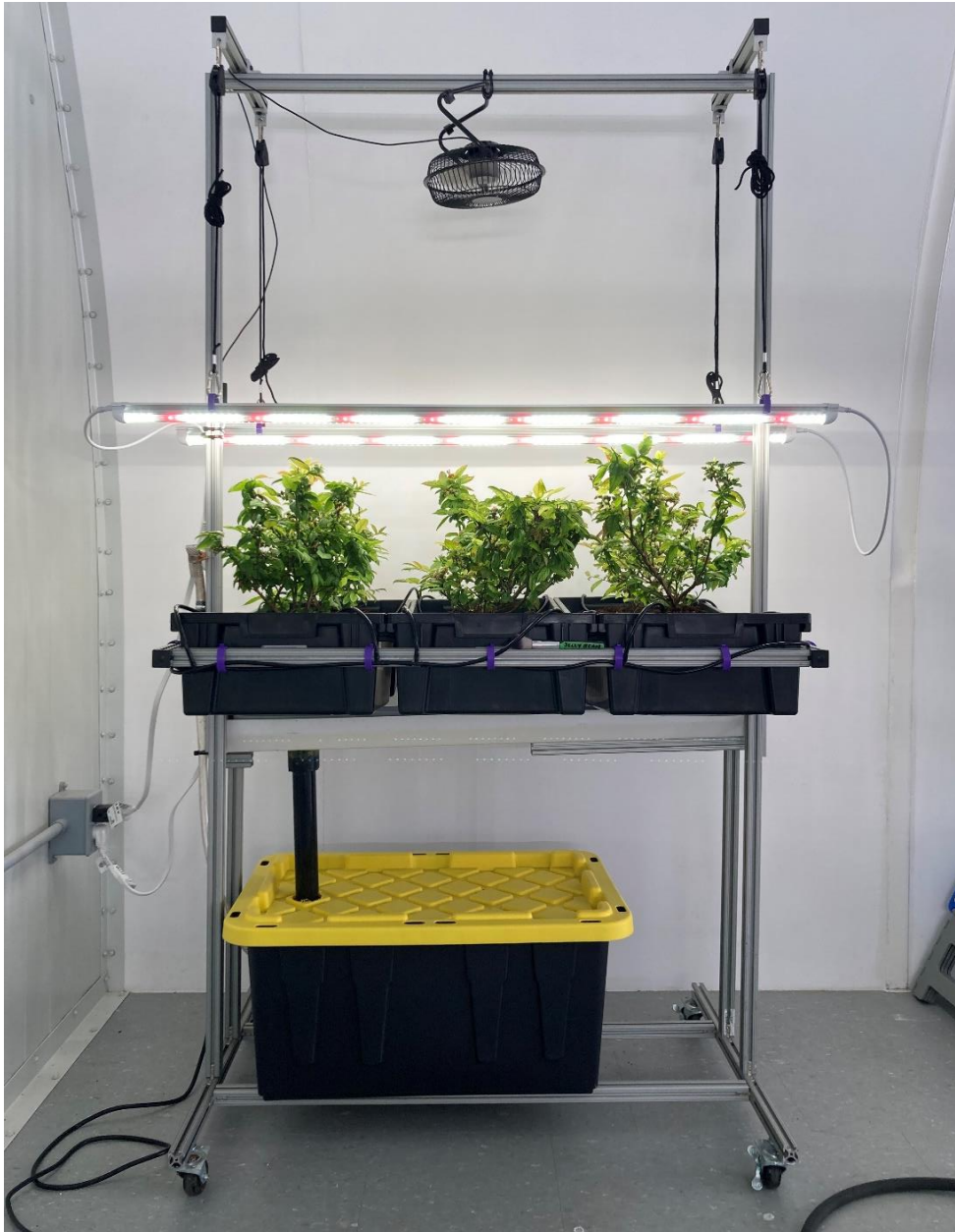
Figure 7. Single water reservoir structure.
