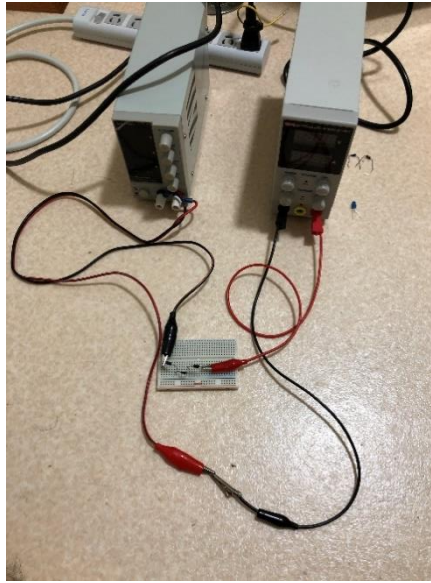
Figure 3-1. The view of the entire circuit (A). Note that the left power supply works as the CC source, whereas the right one operates as the CV source.
