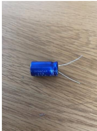
Figure 4. The employed super-condenser. The capacitance is 3.3 F, and the standard voltage is 2.5 V.
