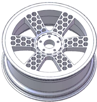
Figure 5. Bionic wheel hub with optimized honeycomb structure.
