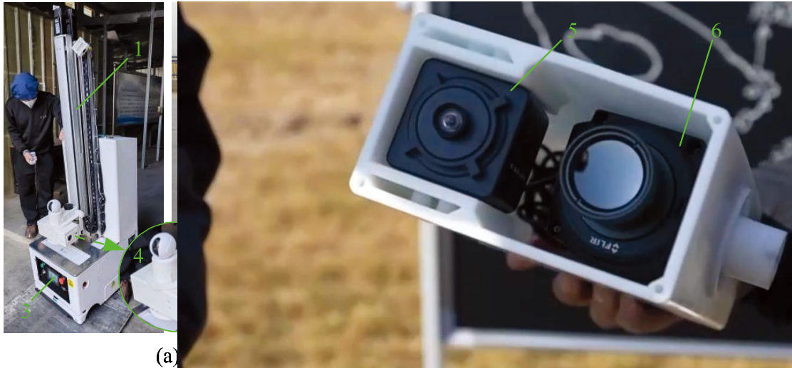
Figure 2. Chicken Inspection Robot. 1, Lifting device of the chicken inspection robot; 2, Information collection and control system; 3, Locomotion device[13]; 4, Monitoring and image capture device; 5, Image capture device - Infrared thermal camera; 6, Image capture device - Visible light camera.
