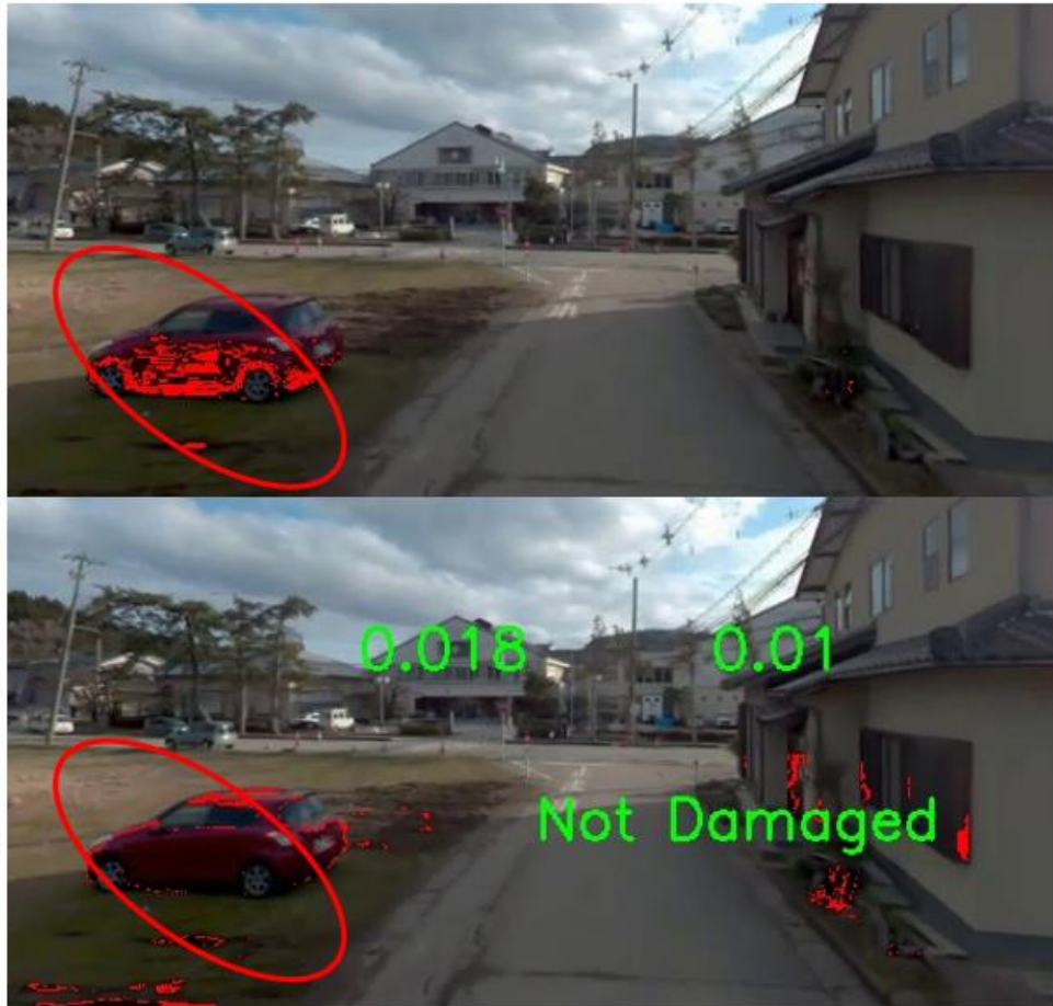
Figure 6. (Top) Example of misidentification as "damaged" by the average of DI (Bottom) An example of correctly identifying "Not Damaged" by the percentage of DI area calibration (the soil in the lower left was misidentified but recognized as "Not Damaged" because it was a small percentage of the total area.).
