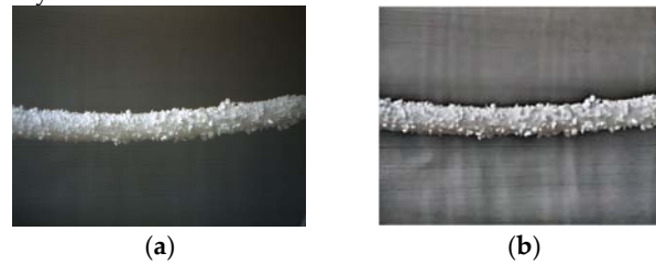
Figure 10. The enhanced image using Multi-Scale Adaptive Retinex and Non-Linear Color Restoration method: (a) The original image; (b) The enhanced image.
