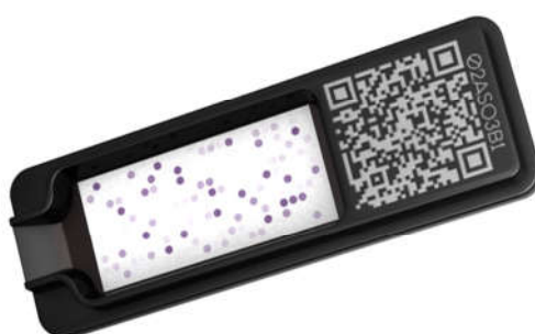
Figure 1. Representation of an ALEX 2 /PAX cartridge, which enables the simultaneous multiplex testing of up to 300 allergens and their controls. Photo courtesy of MacroArray Diagnostics, Vienna, Austria.
