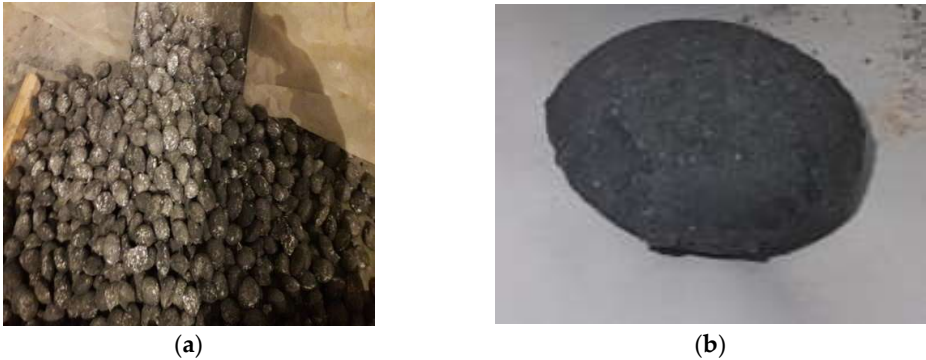
Figure 3. A batch of briquetted monocharge: a - general view; b - briquette.
