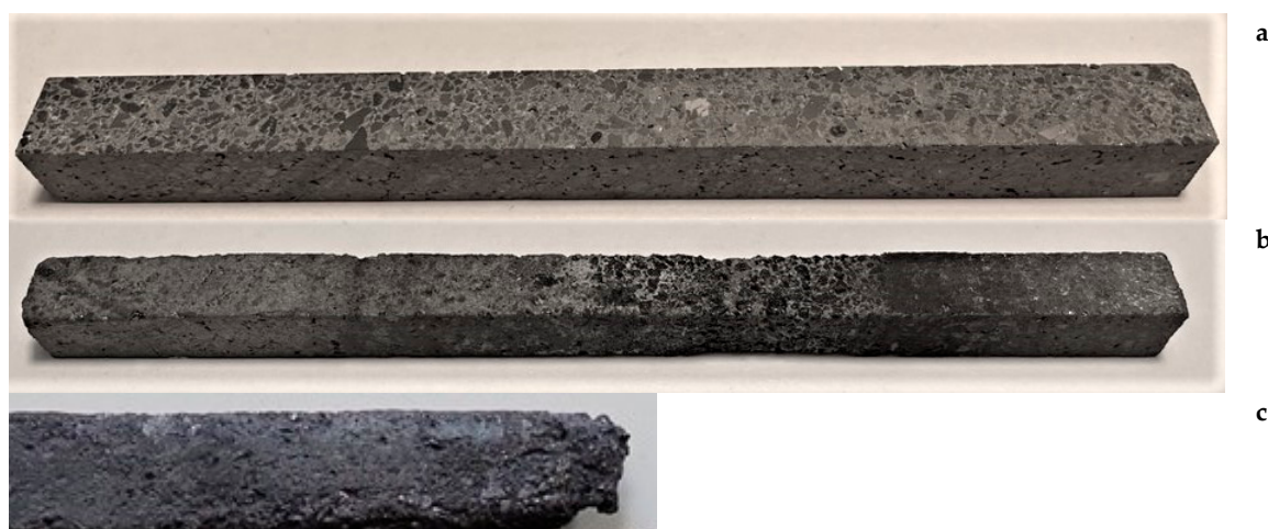
Figure 2. \text{Si}_3\text{N}_4\text{-SiC} rods: a) before lab corrosion testing; b) \text{Si}_3\text{N}_4\text{-SiC} rod after testing, degree of corrosion -2; c) part of \text{Si}_3\text{N}_4\text{-SiC} rod after testing, degree of corrosion -7.
