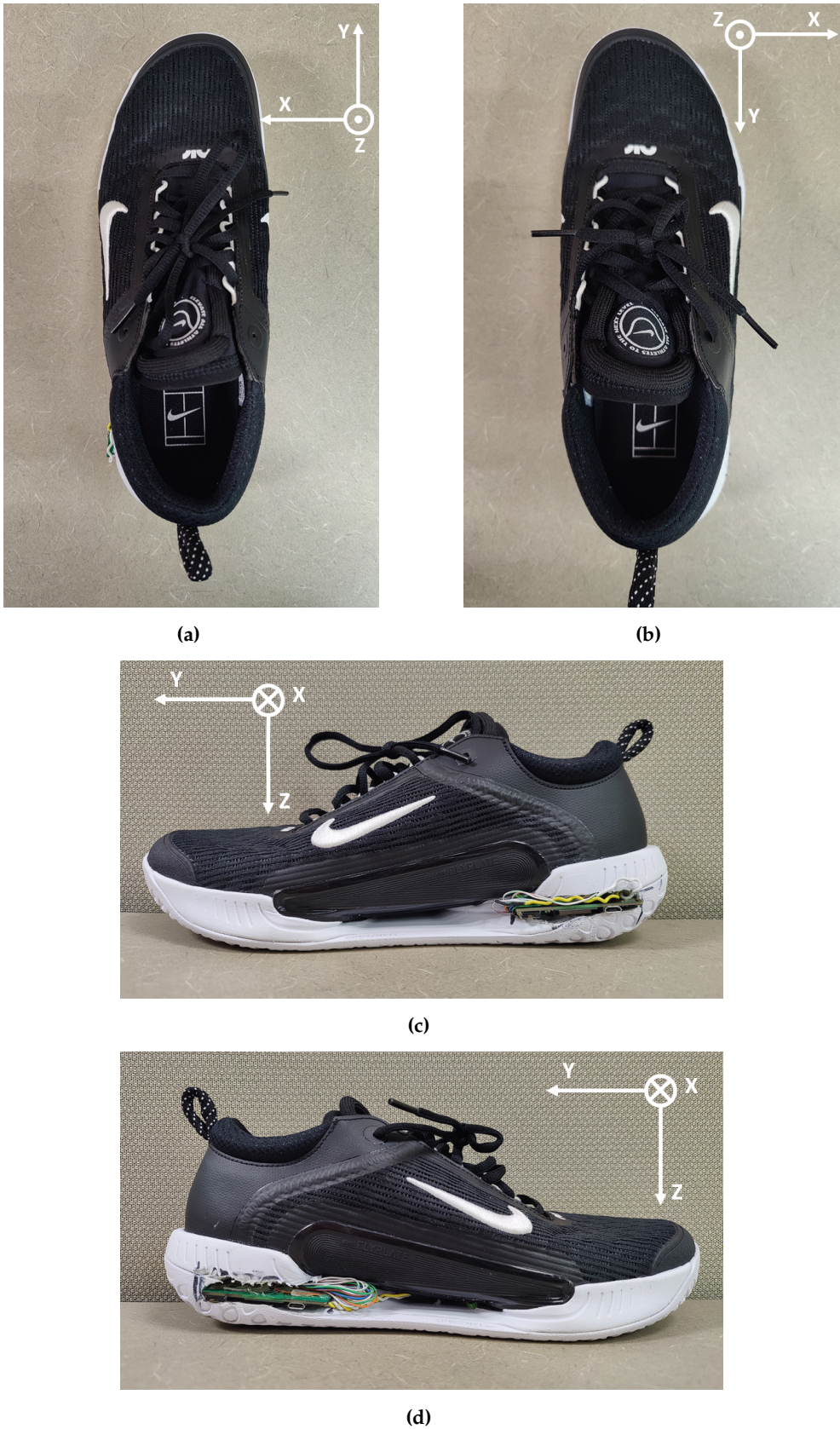
Figure 2. Shoe sensor systems embedded within the shoe soles. (a) Top view of left shoe. (b) Top view of right shoe. (c) Side view of left shoe. (d) Side view of right shoe.
