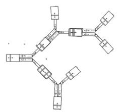
Every MMP unit is fully defined by specifying the position of the piston along its direction of motion, by specifying its rotational state and by specifying the open/close state of all the holes in the piston. This is a time dependent tuple that describes the state of the MMP unit over time. This dynamic tuple defines the applied control strategy. It is perfect raw material for inferential AI neural networks.
