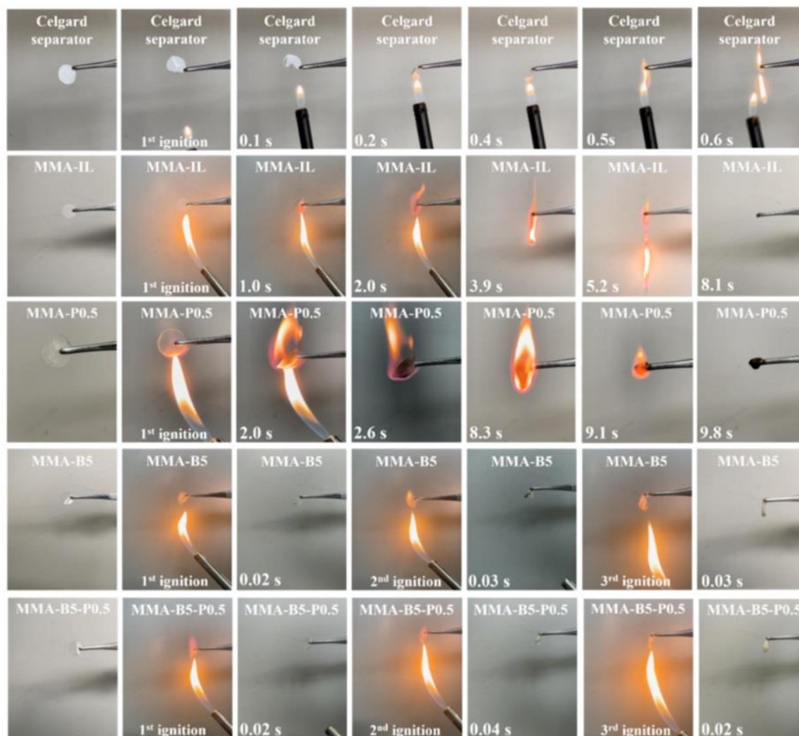
Figure 14. (a) Fire resistance tests for the Celgard separator and GPE films, reproduced with permission from ref. [102], Elsevier.
