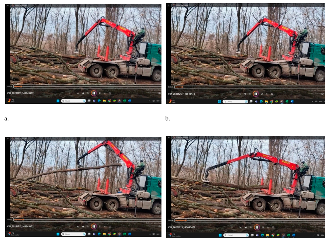
Figure 18. The sequence of working phases from loading wood into a forestry truck: 1 - vehicle preparation (PA); 2 – actuation of the levers that activate the hydraulic arm and the grapple (IPZ); 3 – log measurement (CL); 4 – transfer of the log to the truck/trailer (TBC); 5 – placement/arrangement of log in truck/trailer (AABC); 6 – returning the hydraulic arm and grapple from the truck/trailer to the log (RB); 7 – other activities (AA); 8 – cross-cut technical break (PTS); 9 – getting off the crane after loading (CM); 10 – stop loading by placing the hydraulic arm in the transport position (II).
