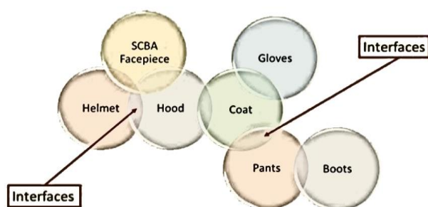
Figure 1. Overlapping interface areas between elements of a structural firefighting ensemble (reproduced with kind permission from [4]).
