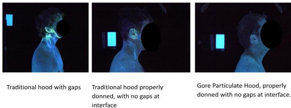
Figure 6. Comparison between traditional hoods and particulate-blocking hoods made from Gore material (reproduced with kind permission from [17]).
