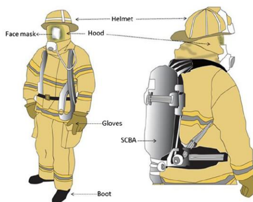
Figure 2. Pictorial representation of firefighter PPE elements (reproduced with kind permission from [6]. © Springer Nature.
