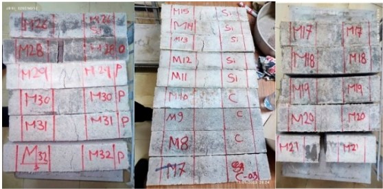
Figure 6. Part of the prisms showing the mode of failure and cracks location.
