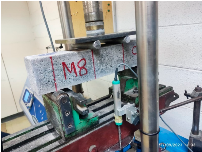
Figure 2. Testing Setup for Evaluating the Flexural Strength and Behavior of FRCC Specimens Using Four-Point Bending Test.
