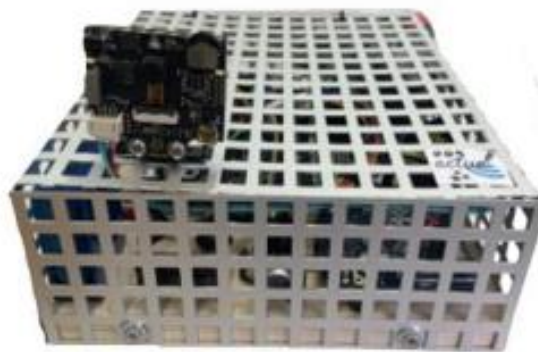
Figure 1. ACTUA Kit device for contextual indoor monitoring.
