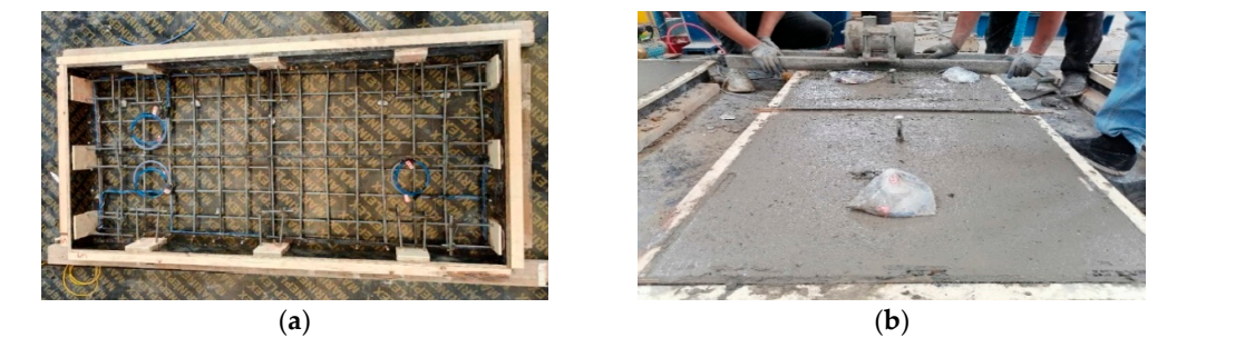
Figure 29. Sensor mounting and plate fabrication: (a) Placement of rebar and (b) Plate leveling.
