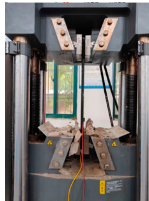
Figure 27. Self-sensing rebar tensile test.
