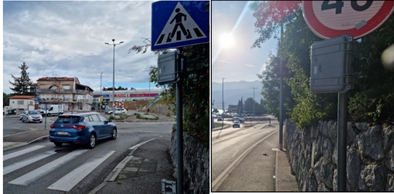
Figure 1. The position of traffic counters: at the entrance/exit from the roundabout (left) and at a distance of 40-70 m from the entrance/exit (right).
