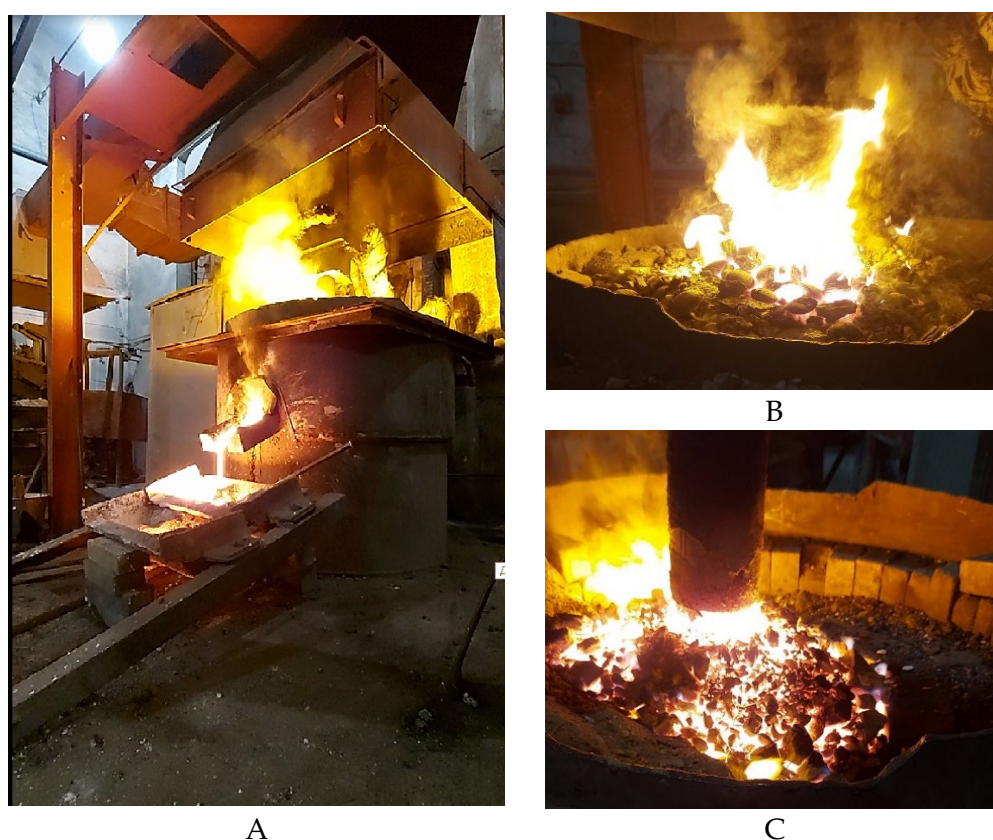
Figure 7. The process of smelting a complex alloy in an ore-thermal furnace with a transformer power of 200 kVA. a - general view of the ore-thermal furnace; b, c - appearance of the flue.
