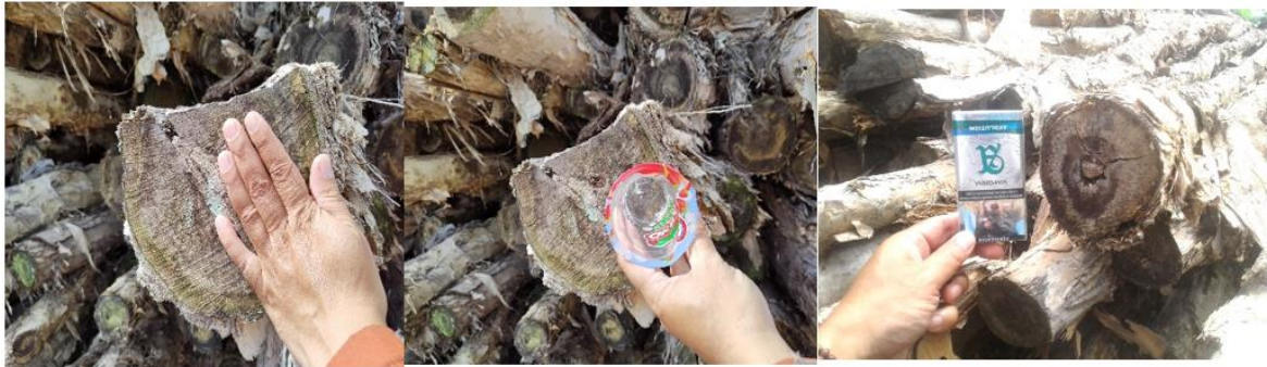
Figure 5. Size of Galam Wood Pile for Foundation.
