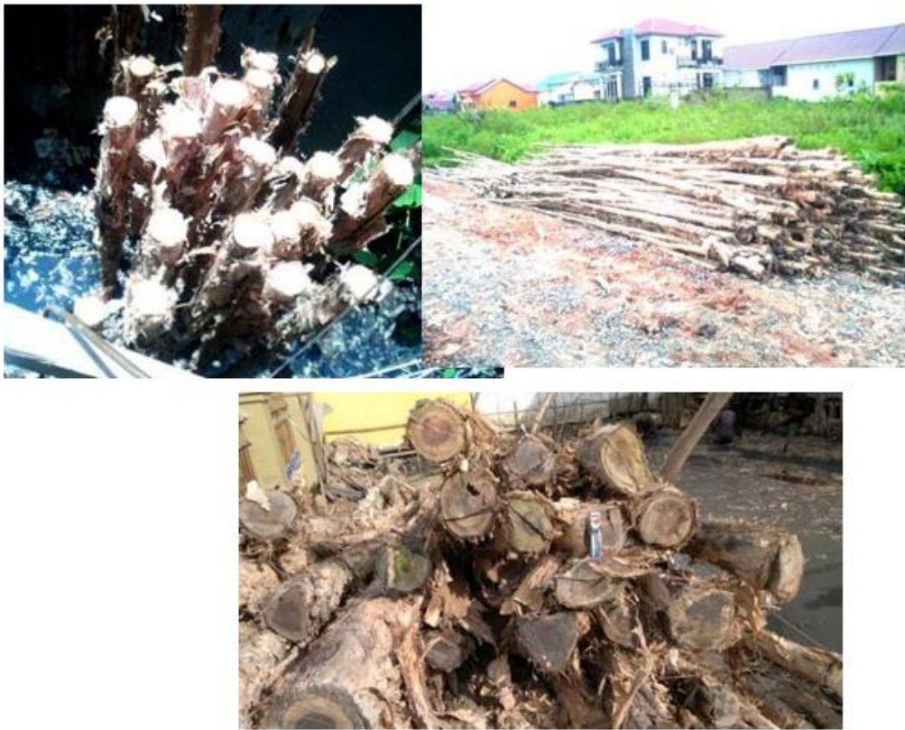
Figure 4. Galam Piling for Foundation.
