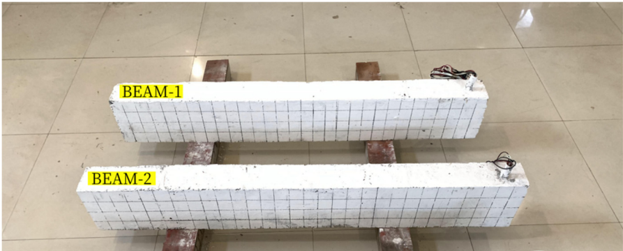
Figure 3. Reinforced concrete beam.
