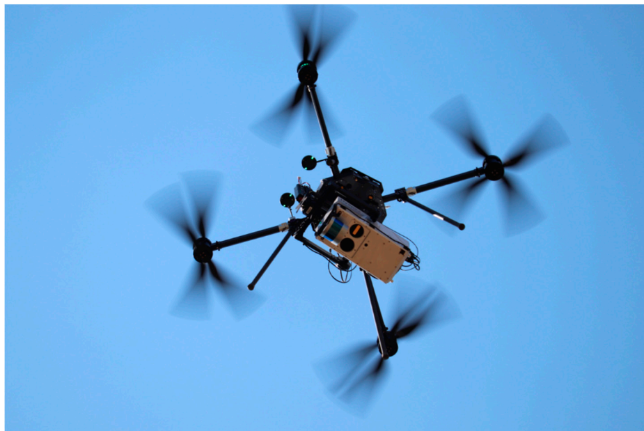
Figure 2. UAS flying the payload of a hyperspectral imager (HySpex Mjolnir VS-620) and LiDAR. Total UAS is below 25kg, size motor to motor 140cm.
