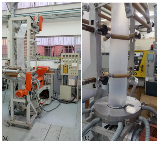
Figure 2. (a) Seibt ES-35 single-screw extruder and (b) blown film.
