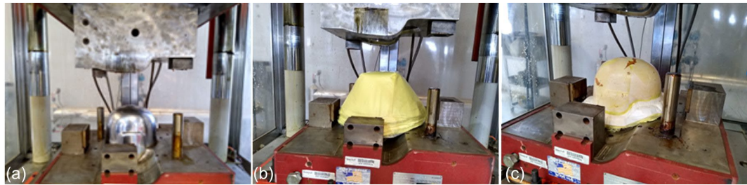
Figure 4. Ballistic helmet pressing: (a) ACH mold; (b) layers of preform in place; and (c) pressed composite.
