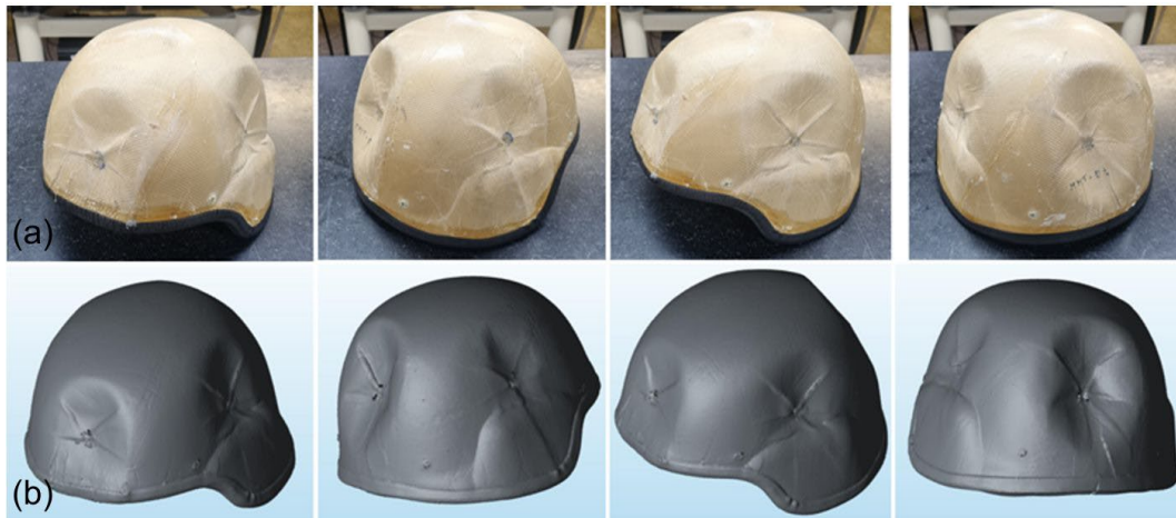
Figure 7. Ballistic tested helmets: (a) HDPE/MMT helmet and (b) 3D reconstructed image.
