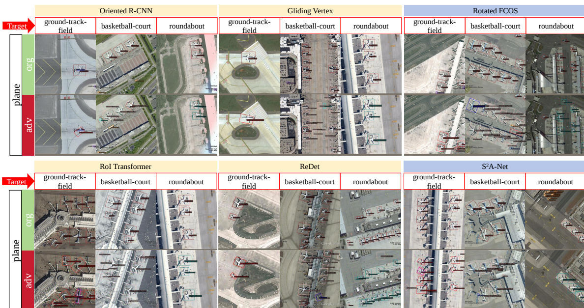
Figure 5. Visualization of object detection results for targeted attacks against planes. The part indicated by the red arrow is the target category, the orange color is the detection result of the two-stage OD, and the blue color is the detection result of the single-stage OD.
