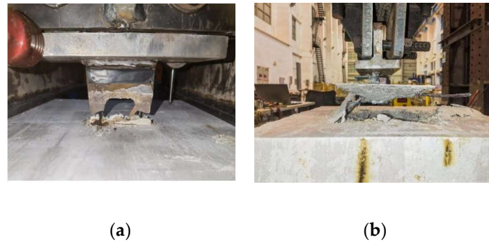
Figure 5. Uplift failures of specimens. (a) Fracture damage of perfobond ribs of PFR; (b) concrete punching damage of PMFR.
