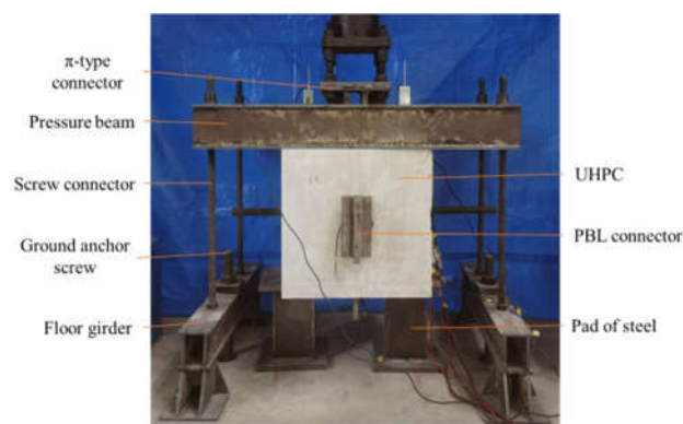
Figure 4. Test setup and instrumentation.
