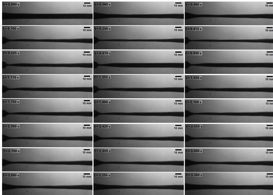
Figure 9. Sequence of images obtained from the first test at a hydrostatic pressure of P_H = 2.943 kPa.)
