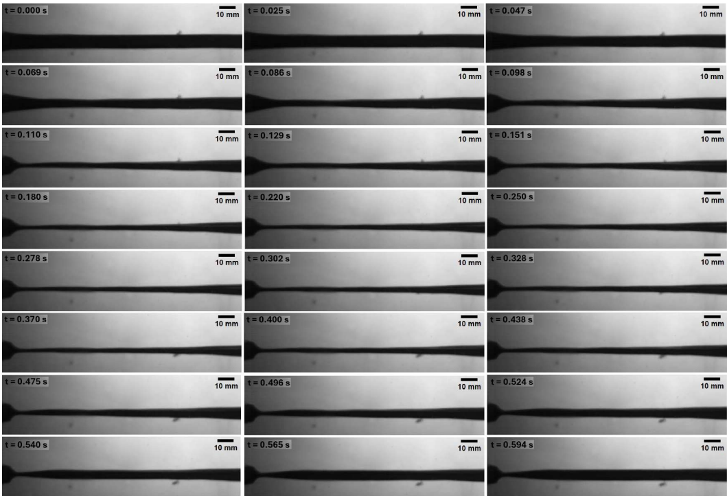
Figure 8. Sequence of images obtained from the first test at a hydrostatic pressure of P_H = 1.962 kPa)
