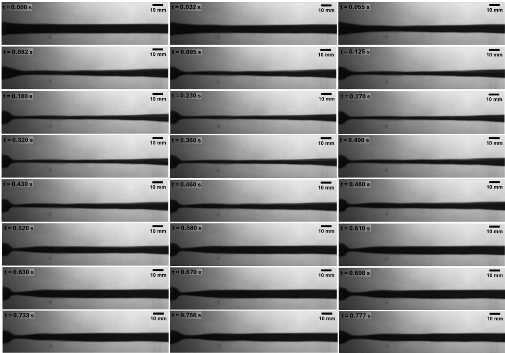
Figure 7. Sequence of images obtained from the first test at a hydrostatic pressure of P_H = 981 Pa)
