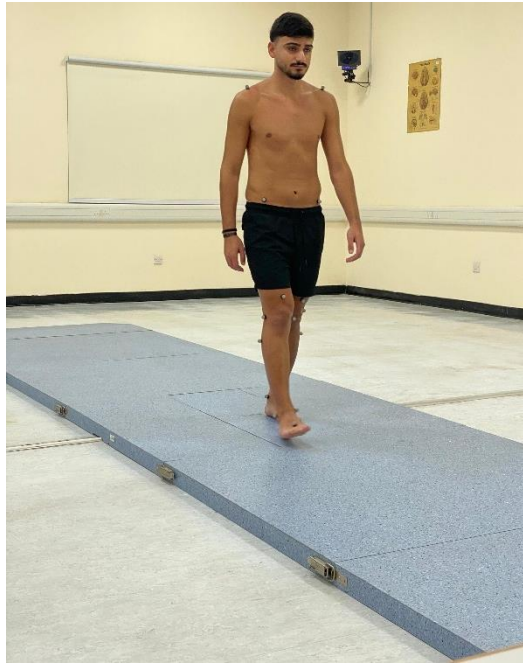
Figure 2. The optical motion-capture system consisting of 8 infrared cameras was used to assess gait kinematics while participants walked along the 10 meter platform. .
