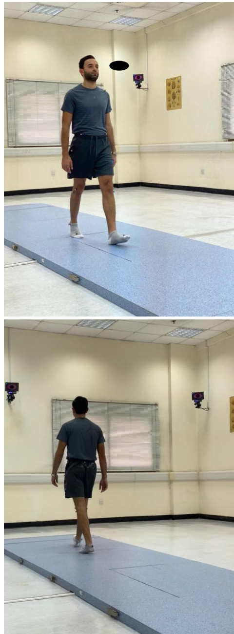
Figure 7. Participants were instructed to walk at their self-selected pace along a 10 m walkway while the 3D trajectories of the markers were captured by the cameras under two conditions: single-task and dual-task.
