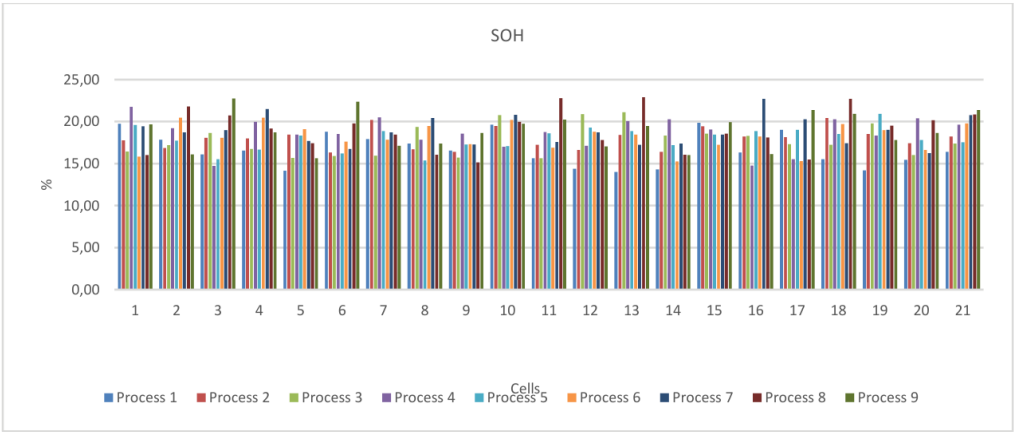
Figure 15. SOH in every cell on each process.
