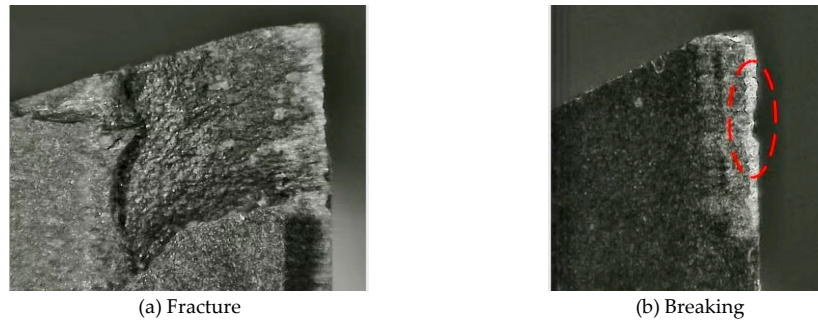
Figure 4. The tool shape after wear.
