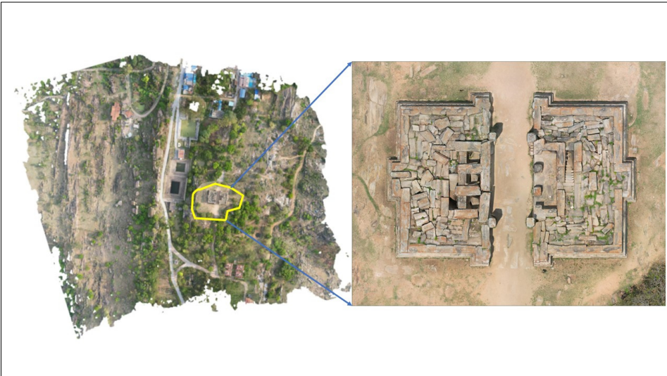
Figure 4. Orthomosaic image output of the aerial survey (left) and zoomed orthoimage of the Raya Gopura (right).
