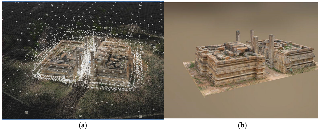
Figure 6. (a) Depicts the camera positions of the Aerial and Terrestrial Camera after alignment; (b) Depicts the final realistic textured model of the monument.
