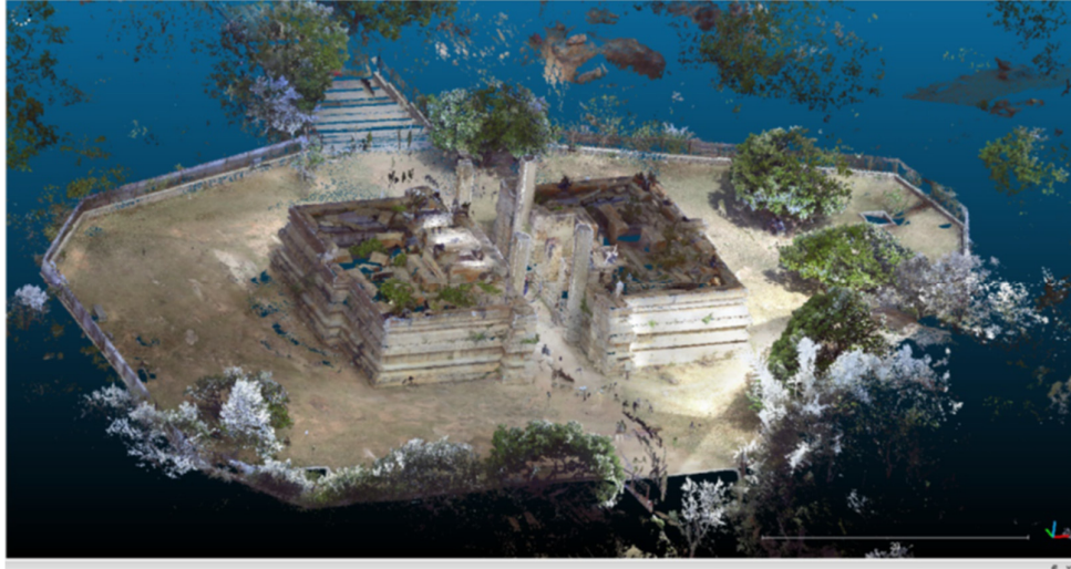
Figure 5. Represents the high density registered TLS point cloud of the monument.
