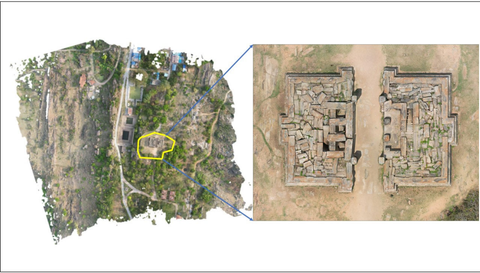
Figure 4. Orthomosaic image output of the aerial survey (left) and zoomed orthomosaic of the Raya Gopura (right).
