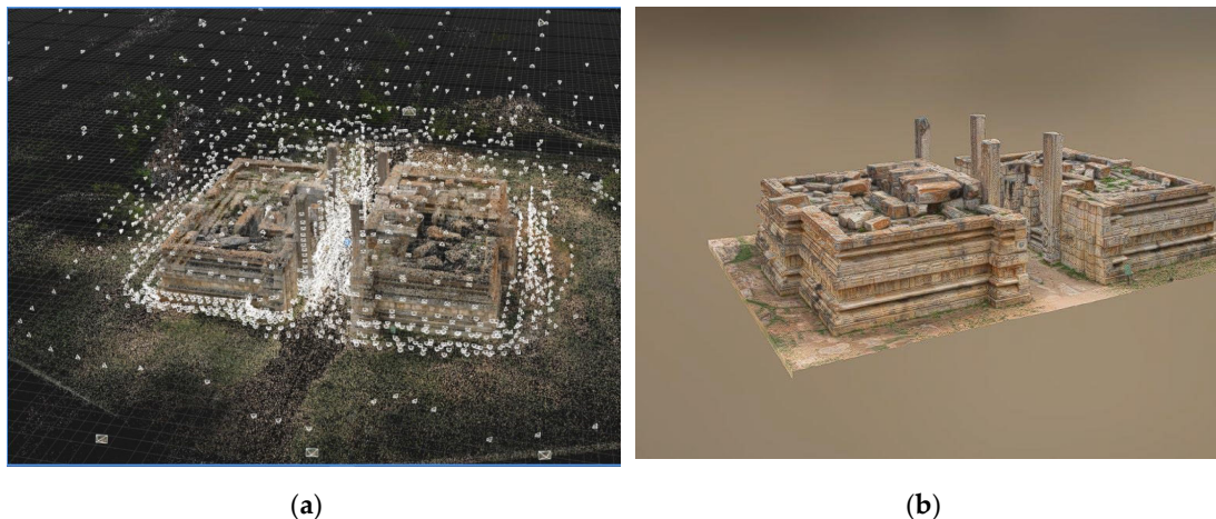
Figure 6. (a) Depicts the camera positions of the Aerial and Terrestrial Camera after alignment; (b) Depicts the final realistic textured model of the monument.
