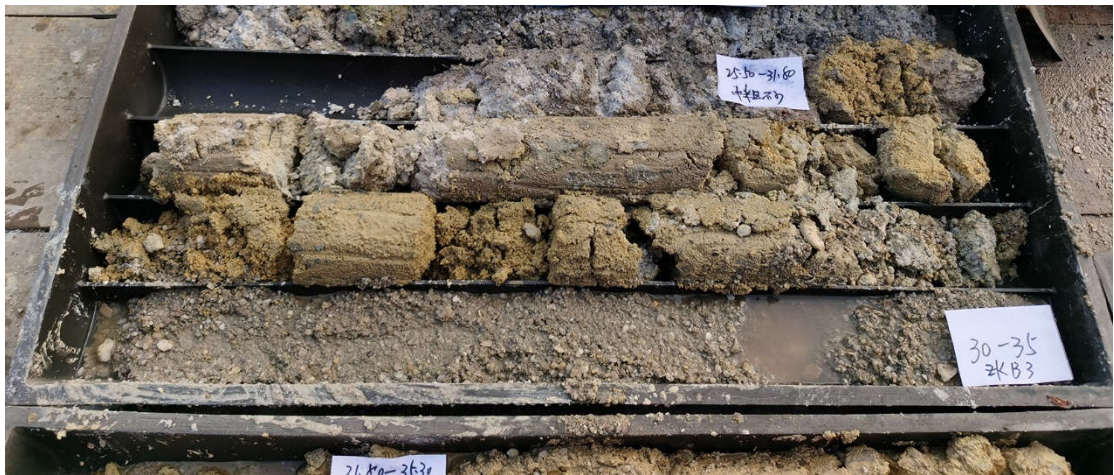
Figure 3. Upper Pleistocene alluvial and proluvial sediment sand layer (YXZK-B3 drilling hole, 30~35m depth).
