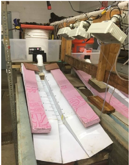
Figure 1. Experimental setup (de-watered) used for the experiments with suckers and chubs at the Saline Research Station. Shown is the ramp with narrow (5 cm) channel.
