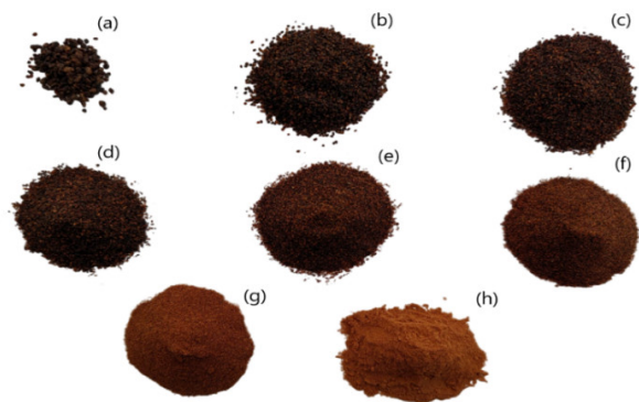
Figure 1. Ground blackthorn berries and the different particle sizes resulting from sieving;(a) >1000µm; (b) 800-1000 µm, (c) 630-800 µm, (d) 450-630 µm, (e) 315-450 µm, (f) 200-315 µm, (g) 125-200 µm, (h) 0-125 µm.
