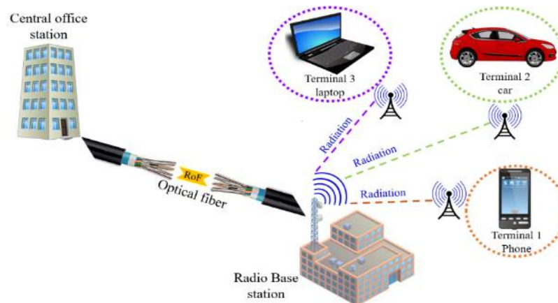
Figure 5. Optical link between the center station and radio base station, wireless links between the radio base station and subscribers.
