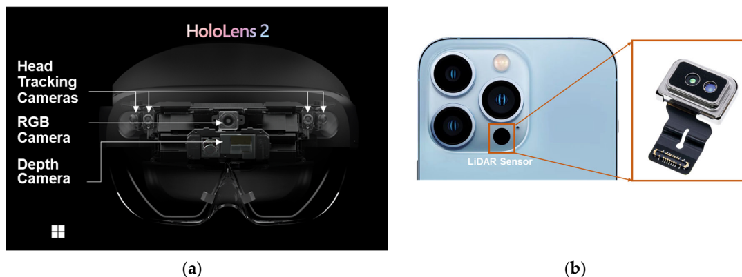
Figure 1. Spatial data collection with built-in depth sensor of MR device (a) Depth camera inside HoloLens 2 (b) LiDAR sensor inside iPhone 13 Pro.
