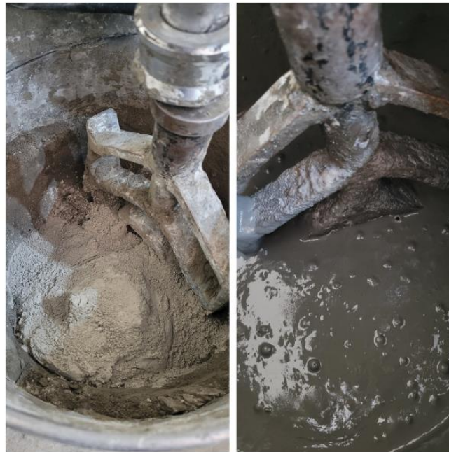
Figure 3. UHPC Mixing Process 1.
