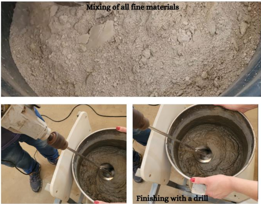
Figure 4. UHPC Mixing Process 2.
