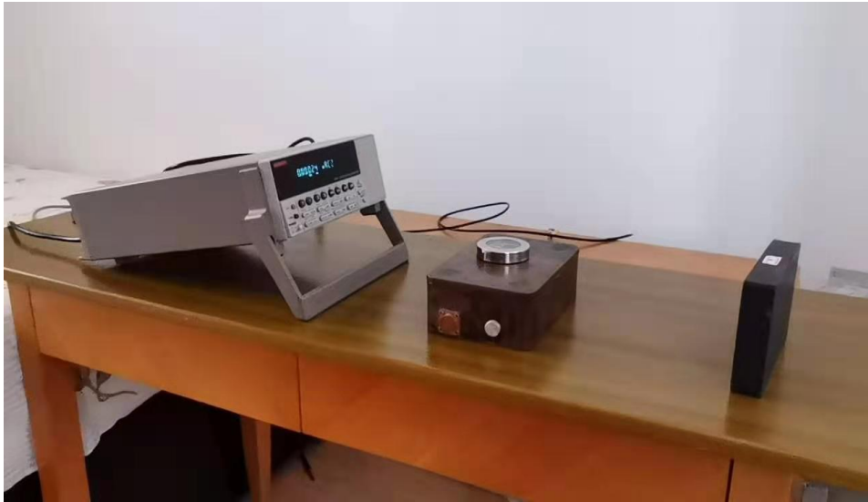
Keithley 6514 ( 10^{-16} \text{ A} ) a copper shielding box a magnet (a) The set up of the experiment (there is a box compass on the top of copper box)
