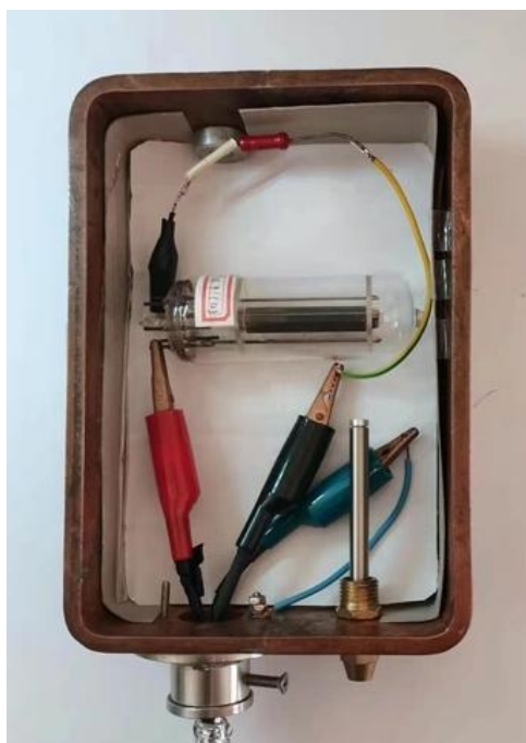
An electron vacuum tube, a resistor R = 150\text{ M}\Omega , some connection lines, etc.
