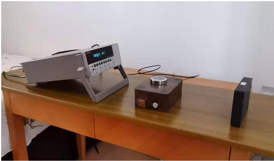
Figure 7. Keithley 6514 (10-16A) copper shielding box magnet.
