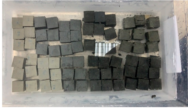
Figure 2. Curing of specimens in water.
